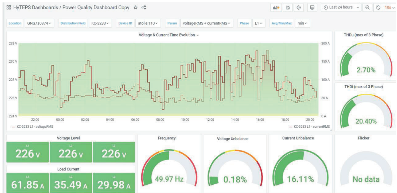
Measurement of power quality and efficient display of results for operation of an installation
